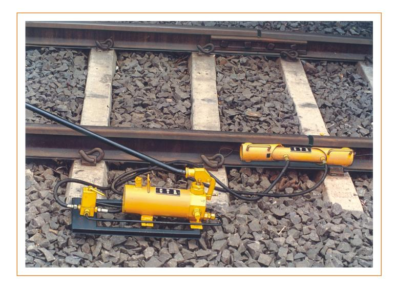
The adjuster alters the longitudinal position of rails, to close or open rail creep. Obstructionless, enabling trains to pass over the track while the equipment is in its working position. The hoses are long enough to allow the hand pump to be kept at a safe distance from the rail. 330mm spigot center distance is suitable for all Broad Guage rail sections. Special spigot center distance for Meter Guage sections on request.
